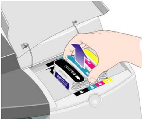
3. Lower the new ink cartridge into its slot until it clicks into place and is quite secure.
