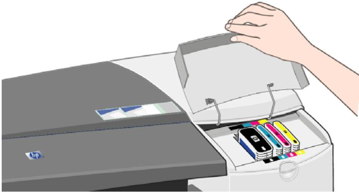
2. Gripping it by its shorter top edges, lift the ink cartridge vertically up and out of the printer.
