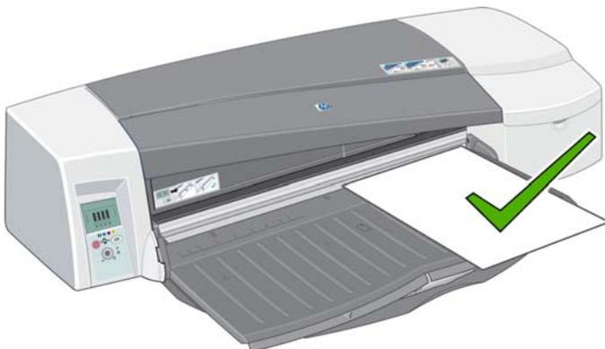
2. If the paper is large enough to hang over the edge of the tray, pull out one or both of the tray extensions to support it.
