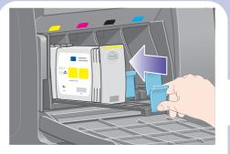
Push the ink cartridge drawer back into the printer until it locks into position.
