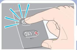
If the power light on the front panel remains off, press the Power key to switch on the printer.
