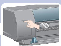
Find the ink cartridge door, which is on the left side of the printer.
