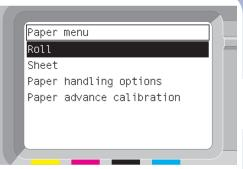
From the front panel, highlight 'Roll' and press the Select (  $\checkmark$  ) key.
