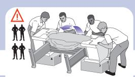
Using four people and the hand holds on the rear of the printer body, carefully lift the printer into an upright position.
