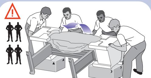
Using four people and the hand holds on the rear of the printer body, carefully lift the printer into an upright position.
