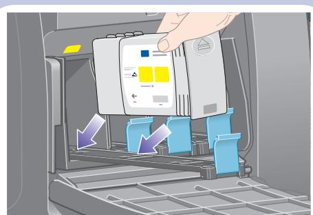
Place the ink cartridge onto the ink cartridge drawer. Note that there are marks on the drawer showing the correct location.
