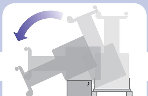
Rotate the printer until its rear rests on the spare and consumables boxes and the wheels with the anti-slip material touch the floor.
