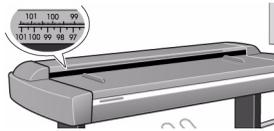
You can change the insertion slot height from 2 to 16 mm (0.08 to 0.63 inches). The Normal position (Step 0: 2 mm/0.08 in) is detected by a sensor in the scanner.
