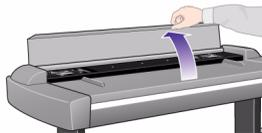
4. Remove the pressure platen.
