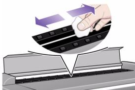
The white scanning area background platen is on the backside of the pressure platen you removed.
