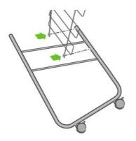
3. Fix the cross frame to the end frame using two screws.
