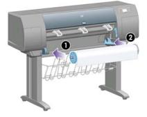
**11.** To make sure that the right end of the spindle is in place, check that the spindle lever is in its top position (horizontal). You can move the lever yourself if necessary.
