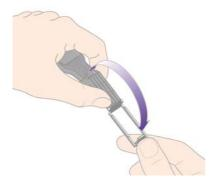
**3.** Load the sponge into the carriage interconnect wiper by positioning the sponge on the face of the carriage interconnect wiper with the shorter tab in the locating slot.
