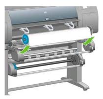
**16.** Lift the drawer 1 paper load lever. This is located on the right-hand side of the printer, above drawer 1.
