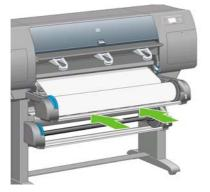
**21.** Using the stops at each end of the spindle, carefully wind the excess paper back onto the spindle.
