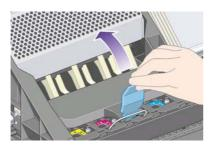
**5.** Before removing the setup printheads, look at the window on top of each one and check that the printhead contains ink. If it does not, contact your customer service representative.
