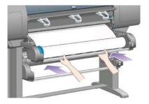
**10.** Wind excess paper back onto the roll. Use the paper stop to turn the roll in the direction shown.
