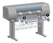
The spindle has a stop at each end to keep the roll in position. The stop at the left-hand end can be removed to mount a new roll, it slides along the spindle to hold rolls of different widths.
