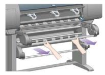
**3.** Load the roll and spindle into the drawer. Hold the roll as shown by the paper stops at each end of the spindle. Try to avoid touching the paper surface.
