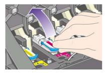
7. Using the blue handle, gently disengage the setup printhead from the carriage.
