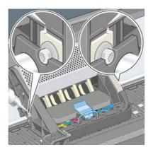
4. Apply a few drops of oil directly to the slider rod on either side of the carriage.
