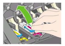
8. Using the blue handle, gently disengage the setup printhead from the carriage.
