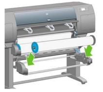
**9.** Lift the drawer 2 paper load lever. This is located on the right-hand side of the printer and under drawer 1.
