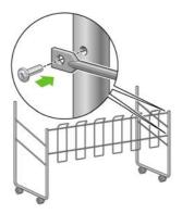
5. Attach the second cross frame to the bin assembly using four screws.
