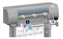
**3.** Remove the blue paper stop (1) from the left-hand end of the spindle. Keep the spindle horizontal.
