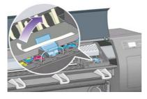
**3.** Pull up and release the latch on top of the carriage.
