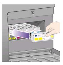
2. When the printhead cleaner has been pushed all the way in, press inwards and downwards as indicated by the arrow shown here, until it clicks into place.
