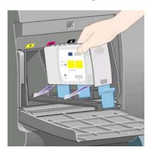
Position the cartridge at the rear of the drawer as indicated below.
