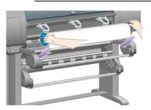
**4.** Lift the paper load lever. Lift the upper lever if you are loading the upper roll, the lower lever if you are loading the lower roll.
