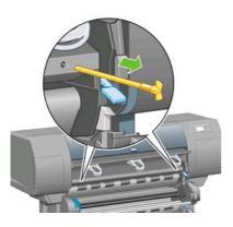
**17.** Remove the two yellow plastic screws from the left and right side of drawer 2.
