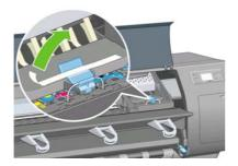
4. Pull up and release the latch on top of the carriage assembly.
