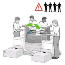
**3.** Rotate the printer until its rear rests on the spare and consumables boxes and the wheels with the anti-slip material touch the floor.
