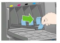
7. Place the ink cartridge onto the ink cartridge drawer. Note that there are marks on the drawer showing the correct location.
