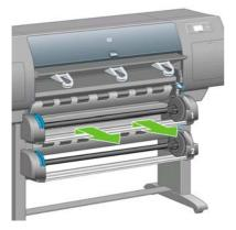
7. Remove the spindle from drawer 1.
