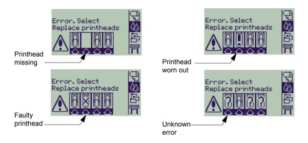
NOTE: An unknown error is displayed when one of the printheads is causing a problem but the system cannot detect which one it is. Refer to Unknown printhead error to solve this problem.
