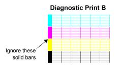
If none of the patterns or blocks in the two **Diagnostic Prints** shows any problem, it could be that your print quality problem is caused by a wrong setting in your software, or perhaps the job should have been printed with the **Print quality** set to **Best** instead of **Normal** or **Draft**.
