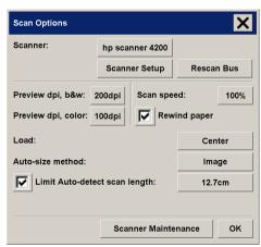
Press the Scanner Maintenance button to start the Scanner Maintenance wizard. The maintenance wizard will guide you step by step through the whole maintenance process: Camera Alignment, Stitching, and Calibration.
