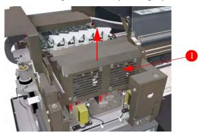
**9** Disconnect the cables from the Head Cooling Fan Assembly.
