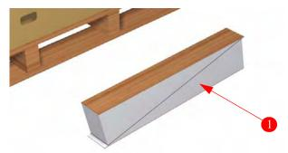
10 Cut the tape on the corners of the cardboard surround at the base of the printer and then, using two people, lift the printer and push in the two Ramps (a little bit at a time) underneath the left hand castor wheels.
