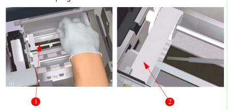
Make sure that the Wiping Liquid does NOT drip onto other parts of the printer. If the Wiping Liquid drips onto the Belt or any nearby sensors, this could cause serious damage to the printer.
