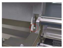
**b** Remove and retain the Hinge from the printer.
