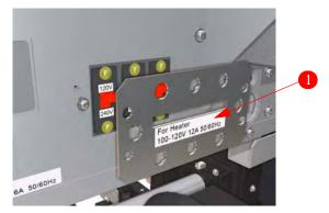
**5** Install the two green screws (1) to secure the Voltage Setting Plate (2).
