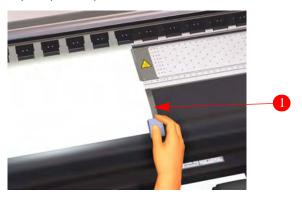
**14** Using the Front Panel, select Roll and press the ✓ key.
