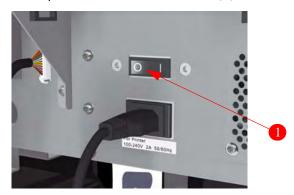
4 Make sure that the Heater Power Switch (1) at the back of the printer is in the Off position and then connect the Heater Power Cable (2).
