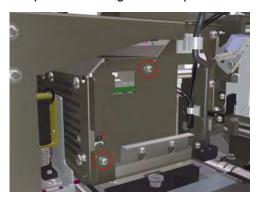
Be very careful when removing the screws from the Head Cooling Fan Assembly as they can easily fall inside the printer.
