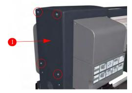
**b** Remove and retain the Right Upper Side Cover from the printer.
