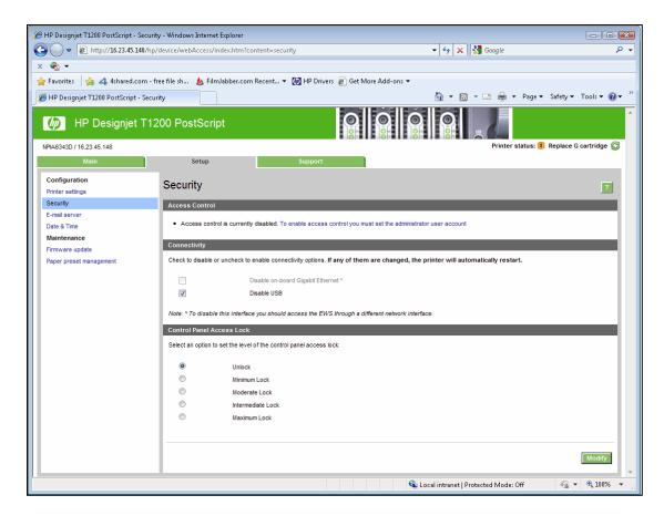
If you enable or disable a connectivity option, the printer will automatically restart. Keep in mind that disabling a connectivity option could cut off network access to the printer. As a security measure, you cannot disable the connection you are using to access the Embedded Web server.
