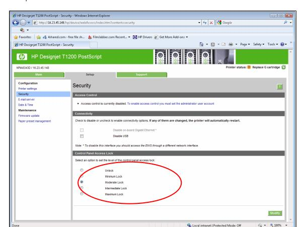
This option can be enabled from the T1200 Embedded Web server as shown below:
